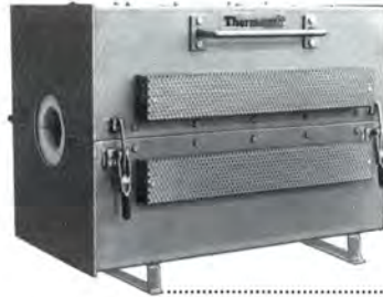
Hinged Split Tube Furnace built to accept 3" I.D. x 24" long ceramic process tube. Three zones of temperature control for maximum temperature uniformity.
